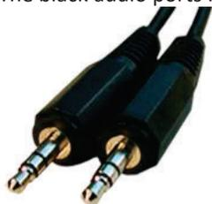
**Figure 11: Audio Loopback Cable**
