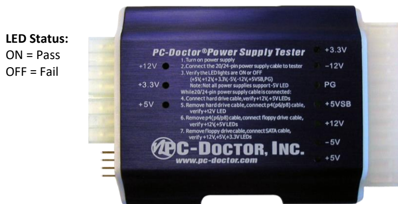
Figure 9: The Power Supply Tester
