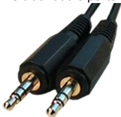
Figure 5: Audio Loopback Cable
