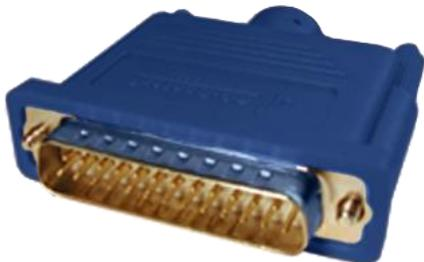
**Figure 6: Parallel Port Loopback Adapter**
